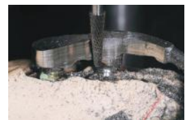
Bar Milling after Casting
