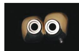
The oxide film is removed by using the Glass bead.
